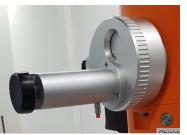
5. Wait until the system reachs a vacuum of  $10^{-6}$  and switch on filament
