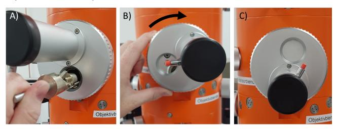
2. Press "Airlock" and immediately turn the knob to the 3 o'clock position while pressing the red button on top of it
